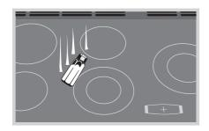
Although the ceramic surface is very strong, a heavy or sharp falling object (a salt cellar for example) might cause the surface to crack. If you find a crack in the surface **immediately** disconnect the appliance from the supply and arrange for its repair.
